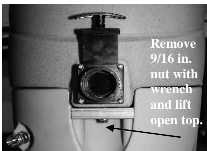
FIG. 4: Solution inlet filter cleaning
