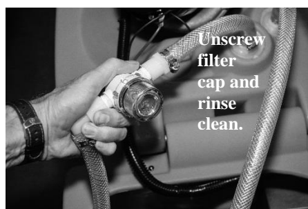
FIG. 4: Solution inlet filter cleaning
